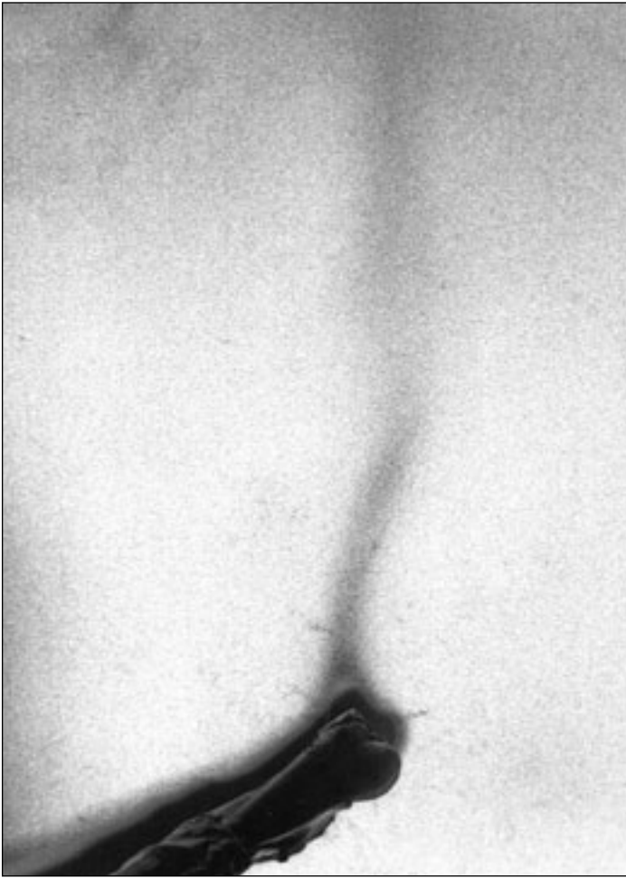
Clouds of mercury vapor are released from a 50-year-old amalgam filling (held in forceps), heated to body temperature (98.6 F) and lightly scratched with a pocket knife (from Reversing Chronic Disease, by Tom Warren).
